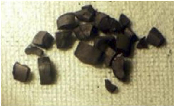
Fig. 1. The irradiated mixed nitride fuel after removing cladding.
